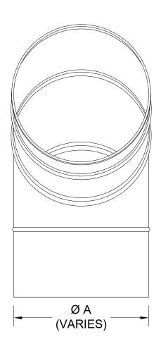
SPIRAL PRODUCED TO SMACNA STANDARDS. CONSULT SMACNA DUCT CONSTRUCTION MANUAL FOR CORRECT GAUGE FOR YOUR APPLICATION.
